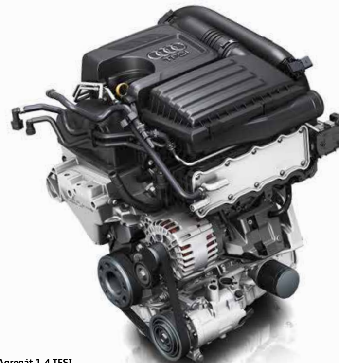
Agregát 1.4 TFSI s technológiou Audi cylinder on demand
