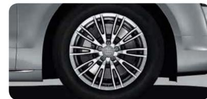
Cast aluminium wheels in 10-spoke V design
