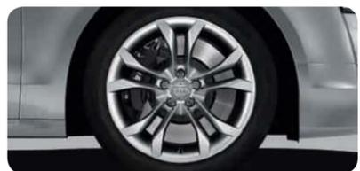
Cast aluminium wheels in 5-parallel-spoke design (S design)
