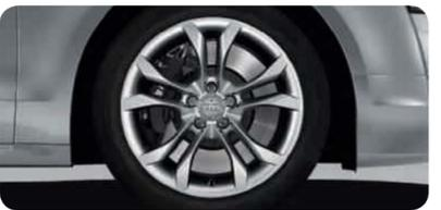
Cast aluminium winter wheels in 5-parallel-spoke design (S design)
