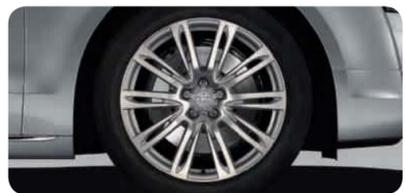
Forged aluminium wheels in 10-parallel-spoke design, partly polished<sup>2</sup>
