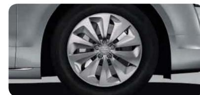
Cast aluminium wheels in 10-arm turbine design (hybrid design)
