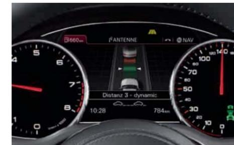
**adaptive cruise control with Stop&Go function including Audi pre sense front<sup>3</sup>**
